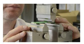
First accredited test centre for CIPP liners in the Netherlands: Material samples from rehabilitated sewers are put through their paces in the laboratory of IKT NL.
