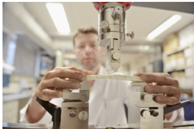
Three-point bending test on a CIPP-Liner
