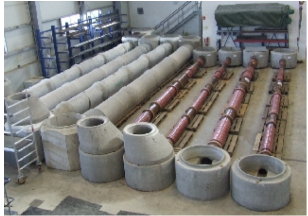
Test apparatus for short-liners and internal sleeves
