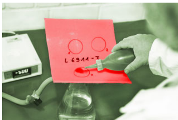
Tight or not? Water tightness test in the IKT laboratory
