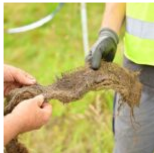
Root mats excavated from the IKT test stand
