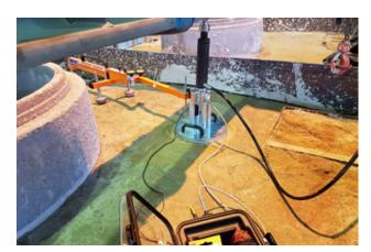
Under pressure: the load plate compression test was used to determine the modulus of elasticity of the installed Flowable Backfills.
