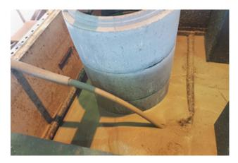
Which flowable backfill best meets the requirements of sewer network owners? IKT has compared five candidates.
