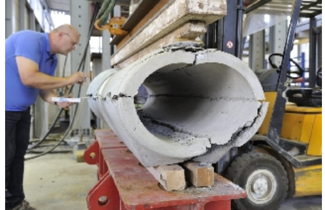
Vertical-compression test on a DN500 reinforced-concrete pipe
