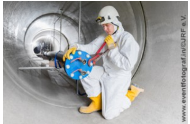
Test rig: IKT research on inspection and condition-surveying of pressure sewer lines
