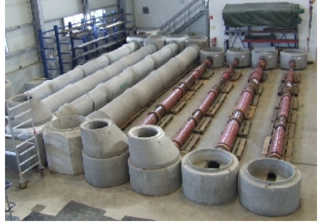
Test apparatus for short-liners and internal sleeves
