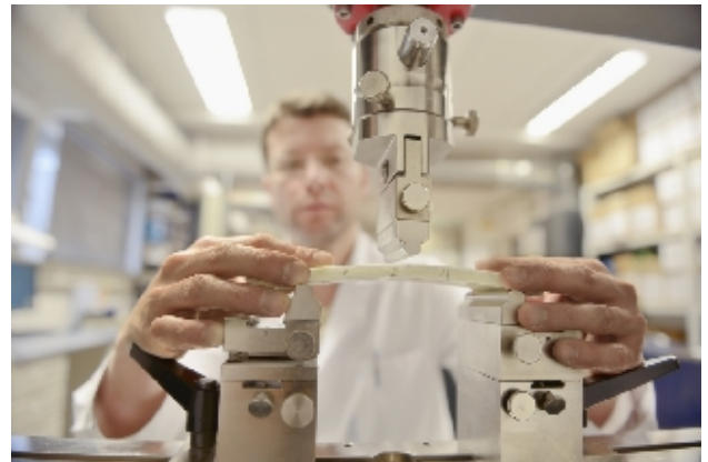
Three-point bending test on a CIPP-Liner
