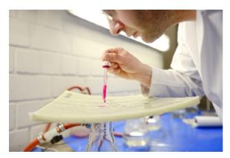
Water tightness: checking if red dyed water penetrates through a CIPP liner
