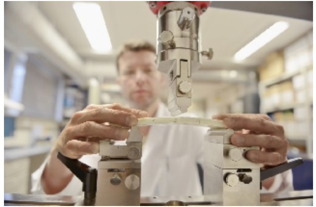
Three-point bending test on a CIPP-Liner
