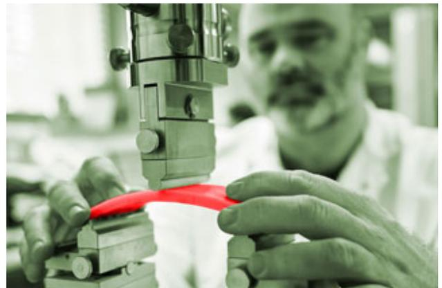
Three-point bending test:
