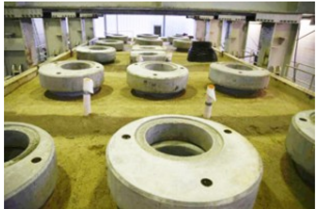
On-site installation conditions simulated in IKT's large-scale test facility
