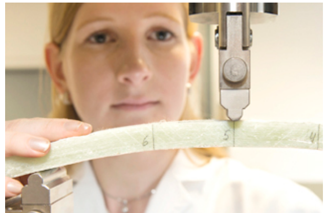
Three-point bending test on a CIPP liner
