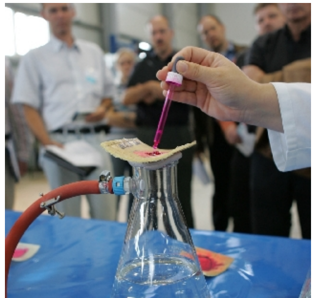
Water-tightness test on a CIPP-liner
