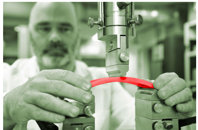
IKT's Test Lab: Three-point-bending test of CIPP sample
