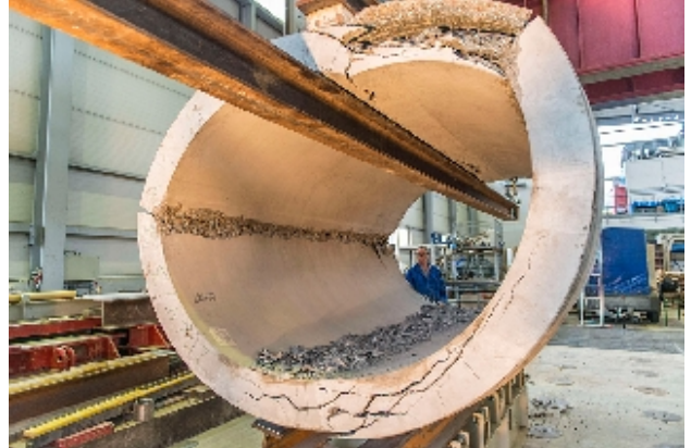
Vertical compression test on a reinforced-concrete pipe
