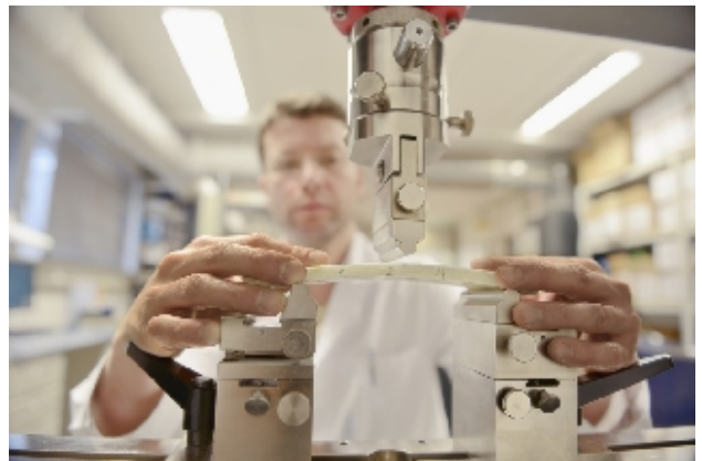
Three-point bending test on a CIPP-Liner
