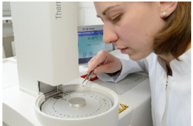
DSC analysis of plastics samples
