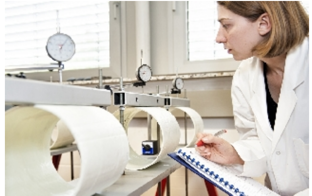
Long-term ring stiffness up to 10,000 h
